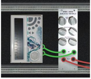
Mixing multiple frequencies before the input, as with this triple VCO, causes them to interact with each other in the distortion, in a way that ranges from subtle added noise to complete trasy chaos. Two frequencies near each other will usually sound somewhat like ring modulation.
