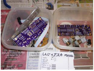
Install wire jumpers at J2 and J4 according to the type of transistors you will install. The Asuka board (left in photo) has PNP transistors, so the jumpers go from the middle hole in each group to the outside (pin 3, round pad, labelled PNP). The Shinji board has NPN transistors, so the jumpers go from the middle
