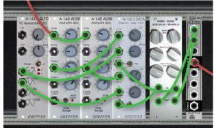
The Asuka and Shinji can be used as a relatively non-distorting amplifier to raise to modular level a lower-level signal such as the headphone output of the Pocket Miku shown here. With appropriate cabling, you can use the two channels for the two sides of a stereo signal.
