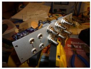
Disassemble the boards from the panel. This step is necessary to free them up for the board-to-board wiring, which couldn't be done earlier because it would have gotten in the way of conveniently soldering the front panel components.
