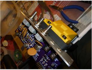
Flip the board and solder the pots and jacks. I used enough solder to fill all the holes in the board, figuring it would provide some structural support, even though that is a fair bit more than necessary for electrical continuity.
