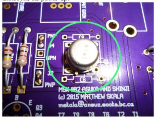
Install the transistors Q1 and Q3 on both boards. These serve as not-very-linear amplifiers, creating most of the "fuzz" effect that is the main purpose of the module.
