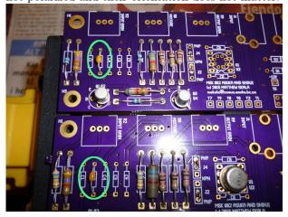
Install the  $22\mu F$  capacitors C5 and C7 on the Asuka board only. These filter the power to reduce transfer of noise from the power supply into the output, though at the lowest output levels some may still be audible.
