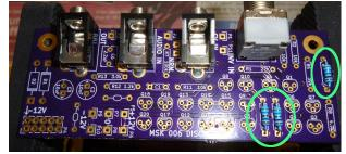
Install the  $1.2k\Omega$  resistor (colour code brown-redred or brown-red-black-brown) R12. This limits the output current.
