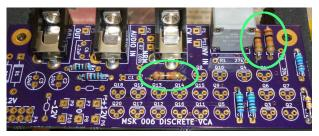
Install the  $27k\Omega$  resistor (colour code red-violetorange or red-violet-black-red) R1. This sets the bias current for the control voltage input buffer.
