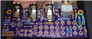
Install the  $100k\Omega$  resistor (colour code brownblack-yellow or brown-black-black-orange) R7. This sets the impedance and limits current on the audio input.
