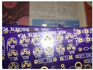
Place (do not solder yet) the jacks and potentiometers in their spots on the PCBs, and assemble the PCBs into a stack using the spacers and threaded hardware. It may be necessary to trim the legs of the potentiometers (just clip 1mm or so off with diagonal cutters—be careful not to remove too much) to get them to fit nicely together.
