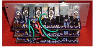
Cut lengths of hookup wire about 8cm to 10cm (3" to 4") and use them to connect P1, labelled "CV IN," on Board 1 to P12, labelled "NRM," on Board 2; and similarly, P1 on Board 2 to P12 on Board 3. This is for CV normalling: each board's CV automatically
