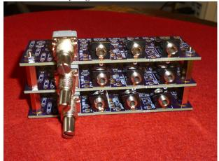
Attach the front panel to the panel components. Screw on all the nuts, but do not use any lockwashers at this time, and only screw the nuts on as tight as you can make them with your fingers. This is only a temporary assembly. The idea is just to hold all the panel components in place while you solder them, so that they will be soldered in perfect alignment with the holes in the panel.
