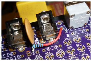
In this photo, I slipped a piece of insulation from a chunk of hookup wire over the resistor lead that goes to P11, so as to reduce the chance of it shorting on other things, and I plugged the capacitor into the pad for R7 nearest P2 instead of actually into the P2 pad, because that made the angle work better. These two pads are directly connected by a trace on the board, so either may be used.
