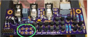
Assemble the stack of boards with the hex spacers, machine screws, and nuts. Attach the front panel, and tighten the nuts on the jacks and potentiometers. This time, use the spring washers and lock washers that came with the pots to make a good, tight installation. Add knobs. You have a finished module.
